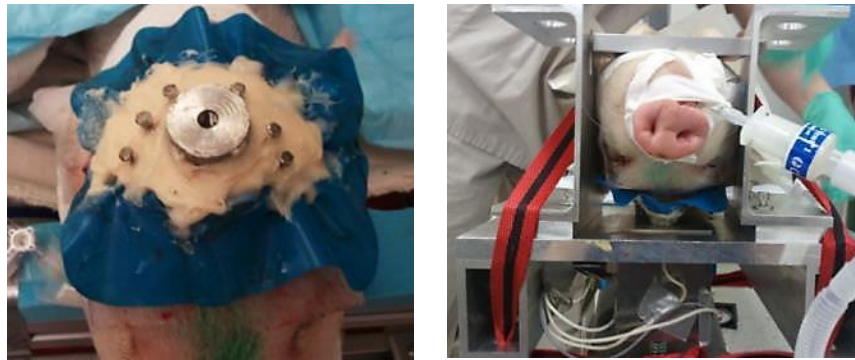
Figure 1: Steel slug and bone screws cemented to the minipig skull (left) and minipig bolted into the injury device and restrained (right).
