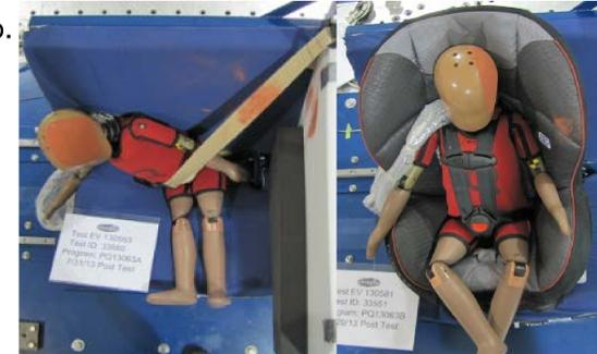
**Figure 2:** a) Schematic for Part 2 of the methods; b) Q3s post-test images from high speed sled test impacts in the lateral direction without CRS (left panel) and in the oblique direction with CRS (right panel)
