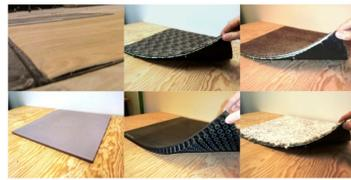
Figure 2: Floor conditions tested (clockwise from top left): Vinyl (V), Commercial Carpet (CC), Residential Carpet (RC), Berber Carpet (BC), SmartCell (SC), Kradal (KR).
