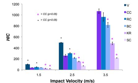
Figure 5: Head Injury Criterion (HIC) scores for impacts across floors and impact velocities. Note: 3.5 m/s impacts not completed on the Vinyl (V) floor
