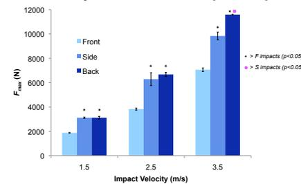
Figure 4: Peak forces following impacts to the front, side, and back of the surrogate headform
