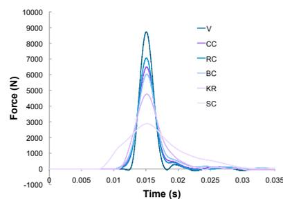
Figure 3: Representative force profiles for 2.5 m/s impacts onto each floor condition (back of the head (B) orientation)
