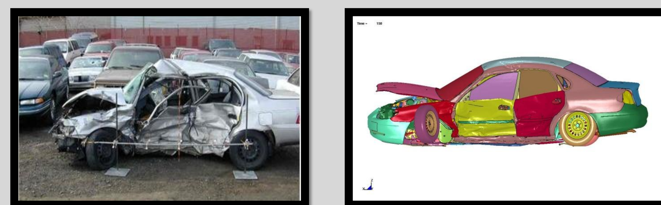
Figure 2: Vehicle deformation patterns of the actual case vehicle and that of the FE simulation using the scaled FE vehicle model
