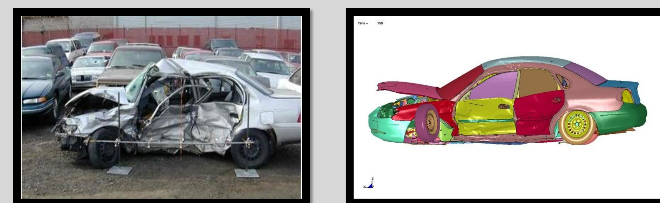
Figure 2: Vehicle deformation patterns of the actual case vehicle and that of the FE simulation using the scaled FE vehicle model
