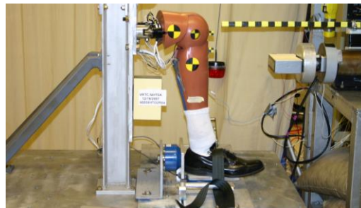
Figure 3: Experimental test setup for impacts of ATD lower limbs
