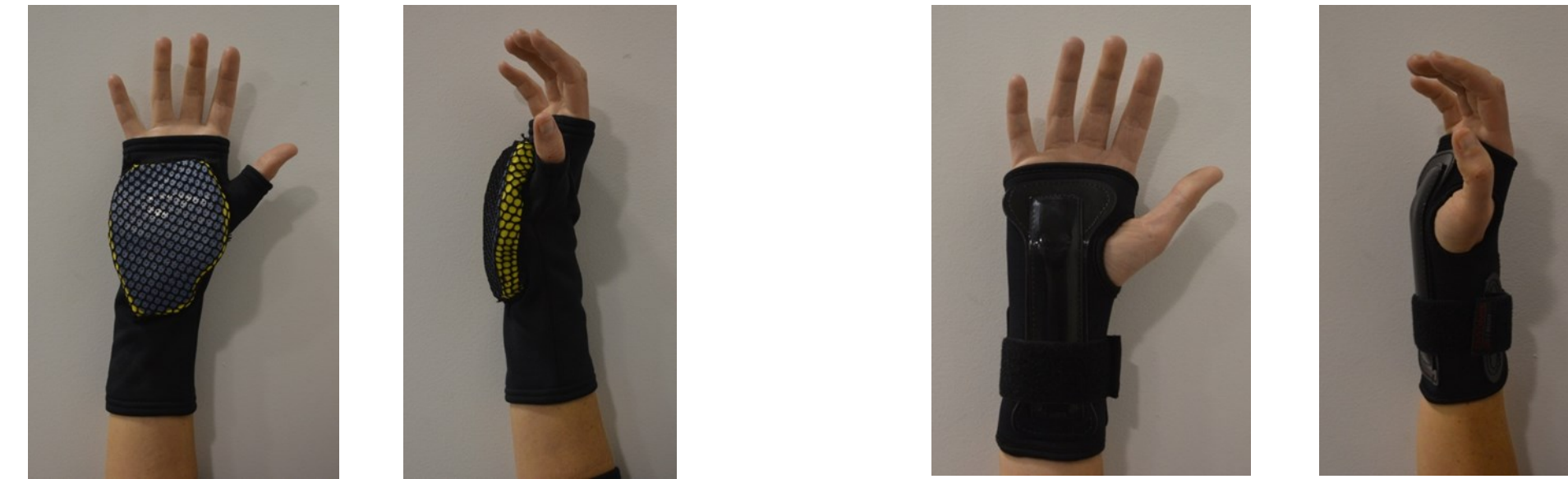
Figure 2: Two different types of wrist guards used in this study: a prototype with viscoelastic foam core and thin rigid shell (left) and a commercially available guard with rigid volar plate (right).
