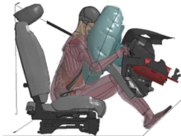
Figure 3: Application of the crash pulse derived from the CIREN case EDR to the tuned SVM.
