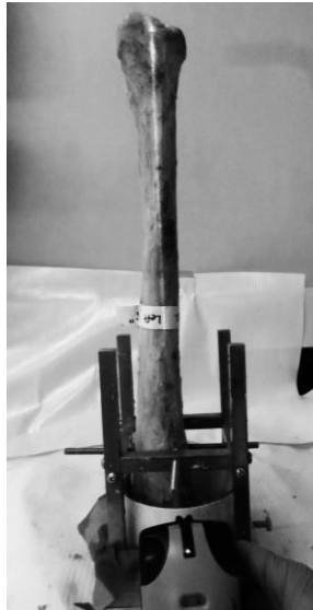
Figure 2: Specimen alignment based on anatomical axes during potting process. The bright vertical line on the specimen is from the laser level used for alignment.
