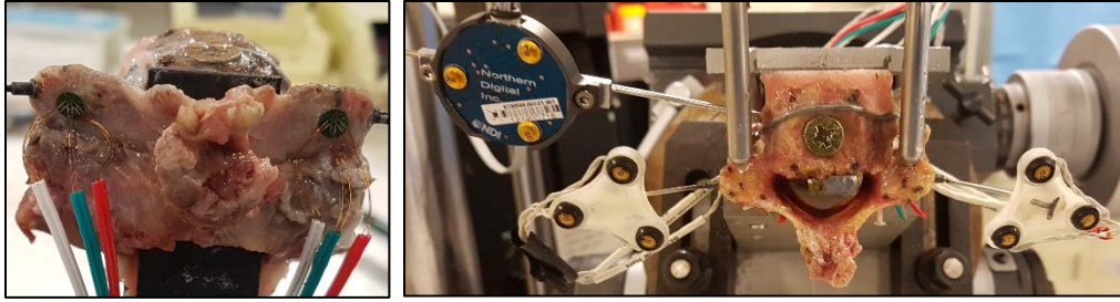
Figure 3: Specimens instrumented with tri-axial rosette strain gauges (left) and custom Optotrak marker-carriers (right).
