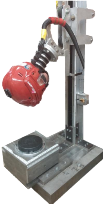
Figure 1: Guided impact tower with helmeted 50 th percentile H-III head and neck mounted on a custom gimbal with a purpose built velocity gate
