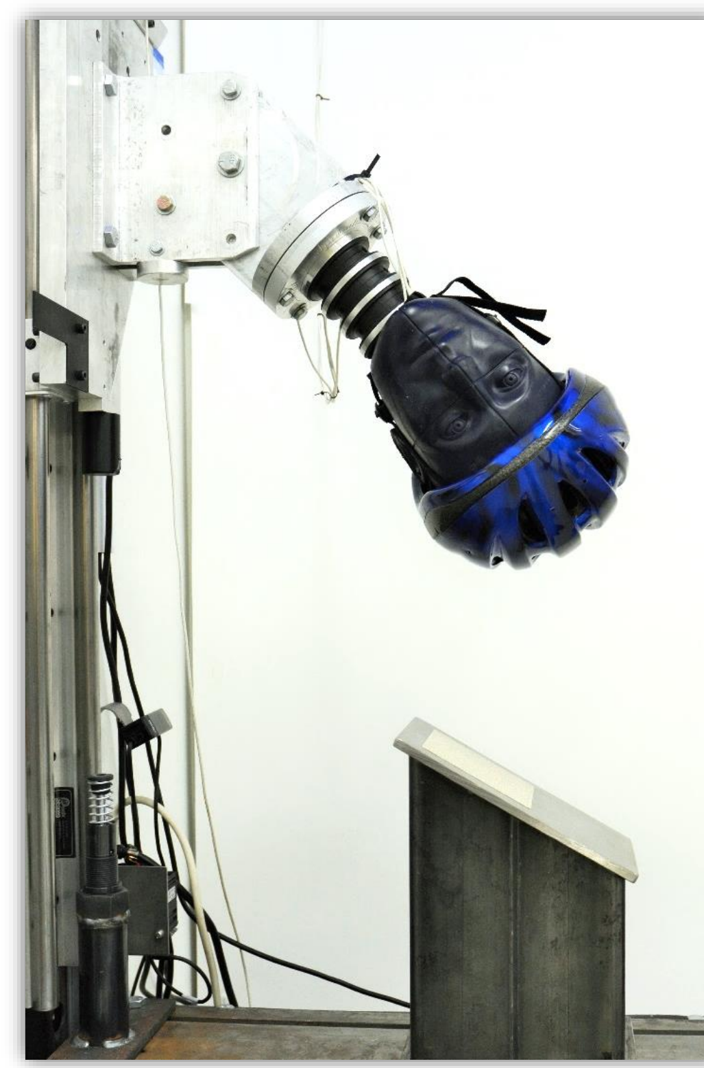
Ten helmet models were impacted on a standard drop rig with a flat anvil and on a custom oblique rig with a 30° anvil.
