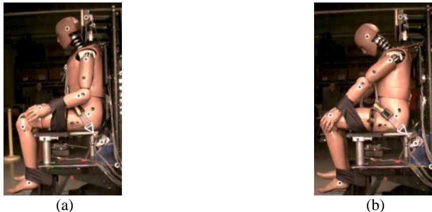
Figure 1: Video still frames from - X, 10G, 70ms rise Hybrid III test. These figures represent the starting position (a) and maximum excursion (b) during the physical test.
