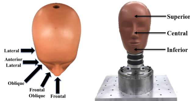
**Figure 1:** The 5 impact directions tested.
