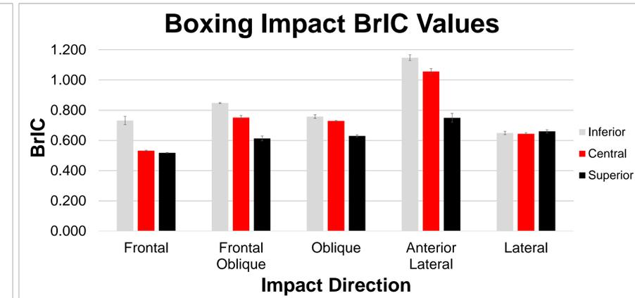
**Figure 5:** BrIC values averaged by impact direction and vertical offset.
