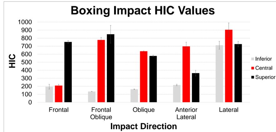
**Figure 4:** HIC values averaged by impact direction and vertical offset.
