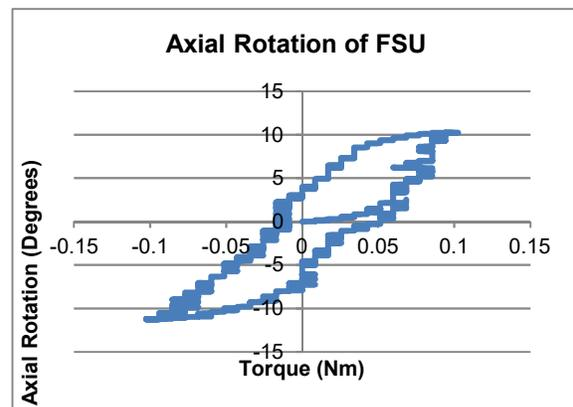
Figure 2 – Sigmoidal Axial Rotation Curve of C3-C5 3D-Printed FSU
