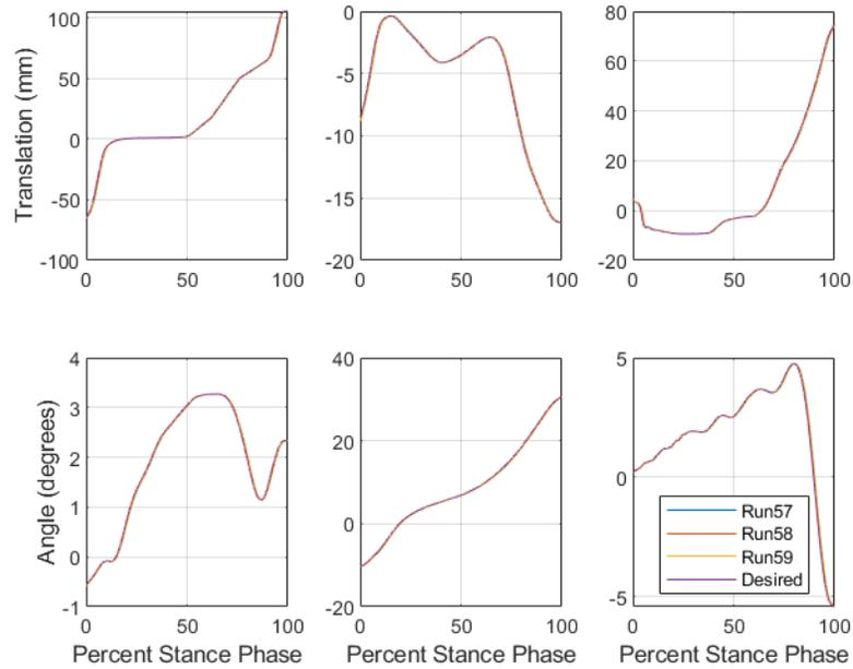
Figure 3: Target Kinematics vs Measured Kinematics in 100% BW condition; Scale is too large to see deviation in the curves; Top row: X-translation, Y-translation, Z-translation, Bottom row: X-rotation, Y-rotation, Z-translation
