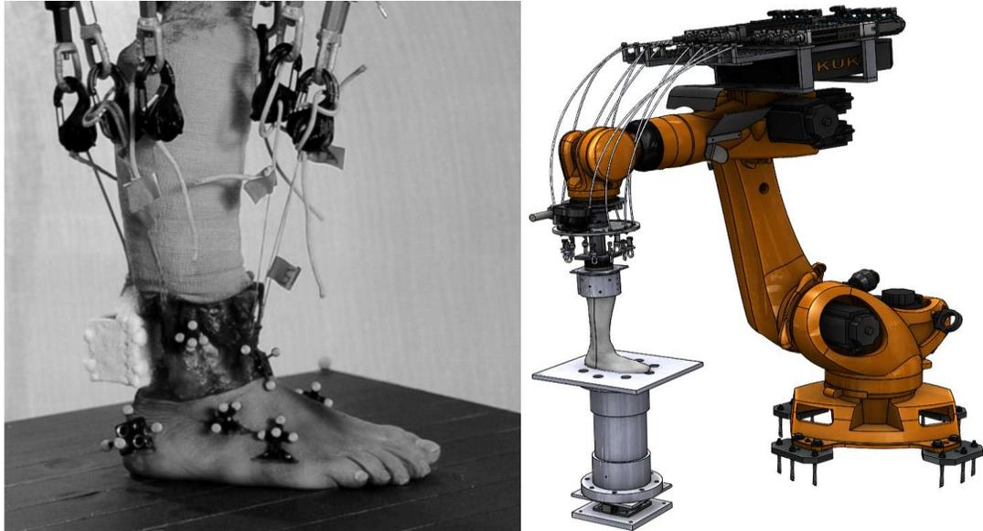
Figure 1: Left –Photo of instrumented PMHS on the MARS. Right – Rendering of MARS.
