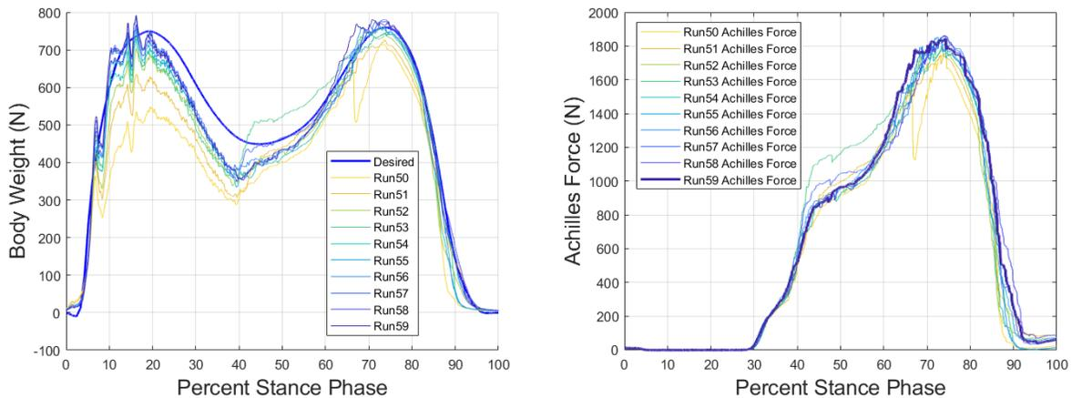
Figure 2: Left- Target GRF vs Measured GRF for multiple optimization runs vs time in 100% BW condition. Right - Demonstration of optimization routine showing Achilles force vs time.
