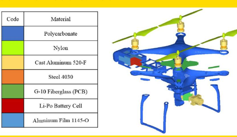
One of the vehicles chosen was the DJI Phantom III, for its high percentage of the sUAS market share. NIAR reverse engineered the Phantom III to created a virtual FE model.
