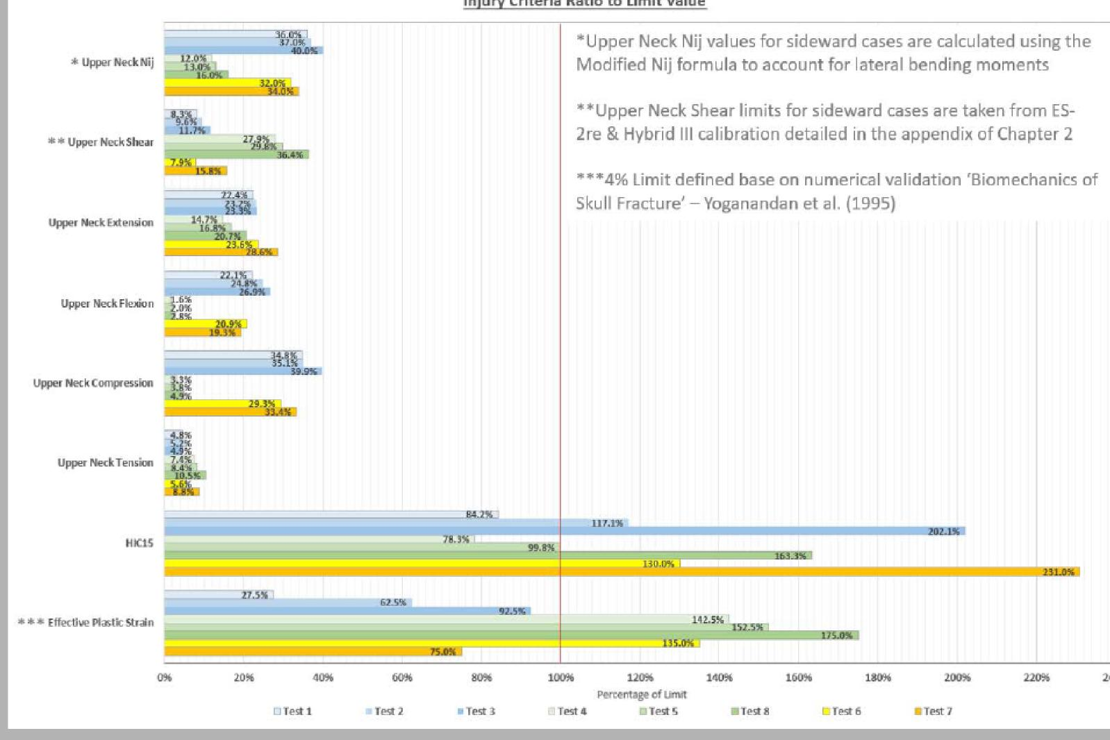
case orientation. The additional injury criteria and skull strain evaluation showed a high probability of skull fracture for the front first, angled forward impact. There were some high strains and fracture potential also noted for the front first, 0° to side of head, impact. However, the specific modeling method of the ear structure for the THUMS was considered to be unrealistically enduring this fracture.
