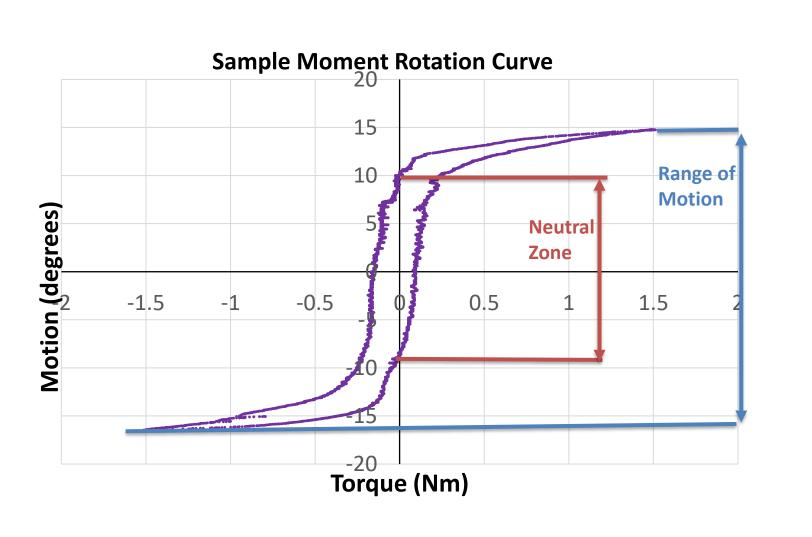
Range of motion is presented in the darker colour and neutral zone in the superimposed lighter colour. The results of this study are in red
