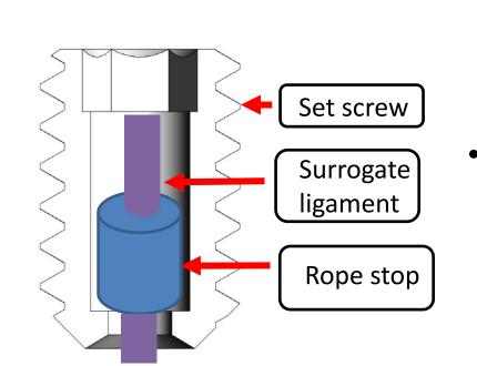
Ligament tension was set by using a torque limiting screw driver to tighten set screws with the surrogate ligament material inset
