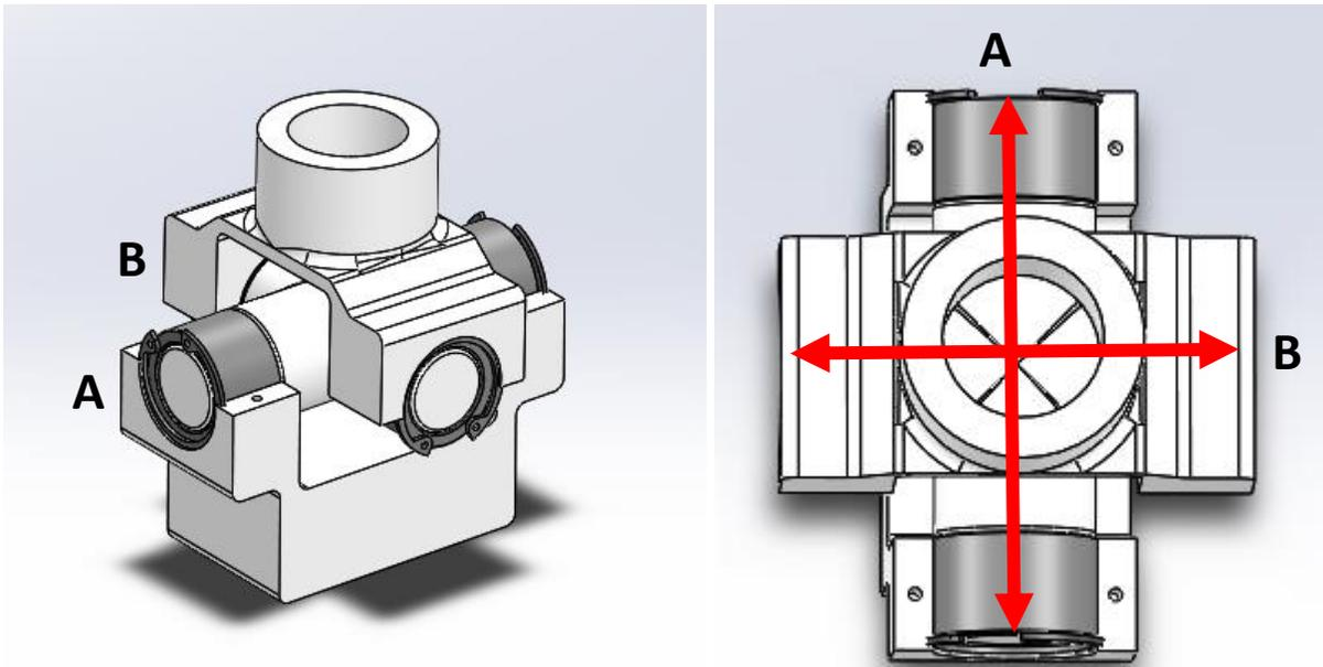
Figure 3: 3D printed universal joint for prototype version 3. A) Anatomical equivalent for ankle length B) Anatomical equivalent for bimalleolar width
