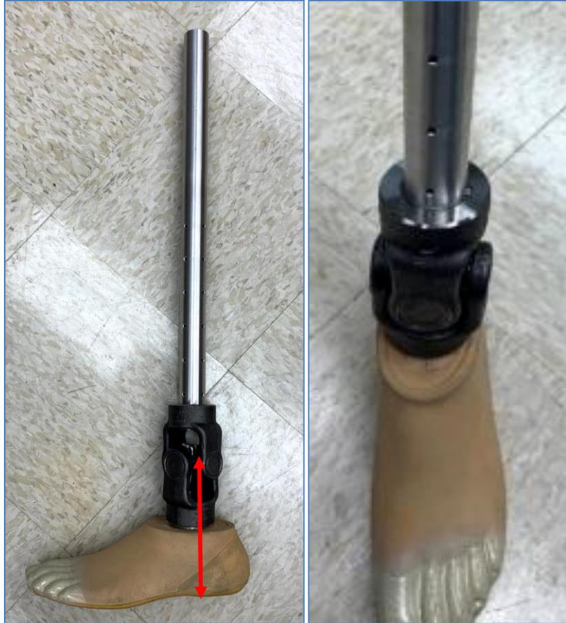
Figure 1: Surrogate prototype version 1. Lateral view with arrows indicating universal joint center of rotation and top view close up.
