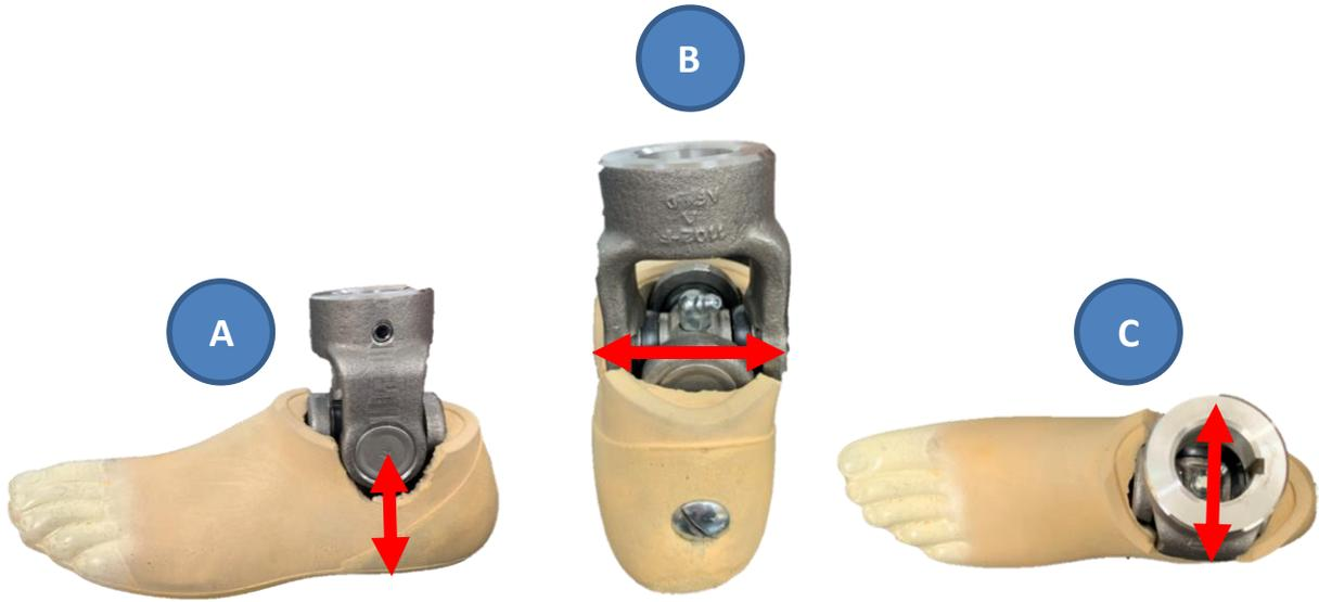
Figure 2: Surrogate prototype version 2. A) Lateral view arrows indicating center of rotation equivalent at lateral malleolus B) Posterior view arrows indicating anatomical equivalent bimalleolar width C) Top view arrows indicating anatomical equivalent bimalleolar width
