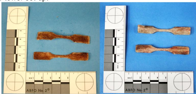
Figure 2: ASTM D638 Type V dog bone samples for high-rate testing
