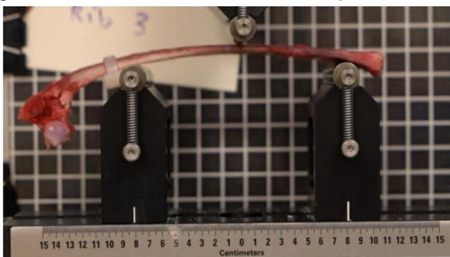
Figure 1: Three-point bend mechanical testing set-up for rib mechanical testing
