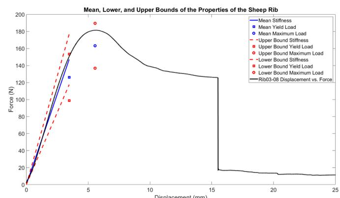
Figure 4: Mean force-displacement curve and properties of quasi-static tests
