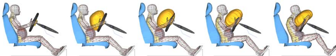
The response of the pregnant occupant model in a frontal impact case with airbag and no seat belt for 20 ms intervals
