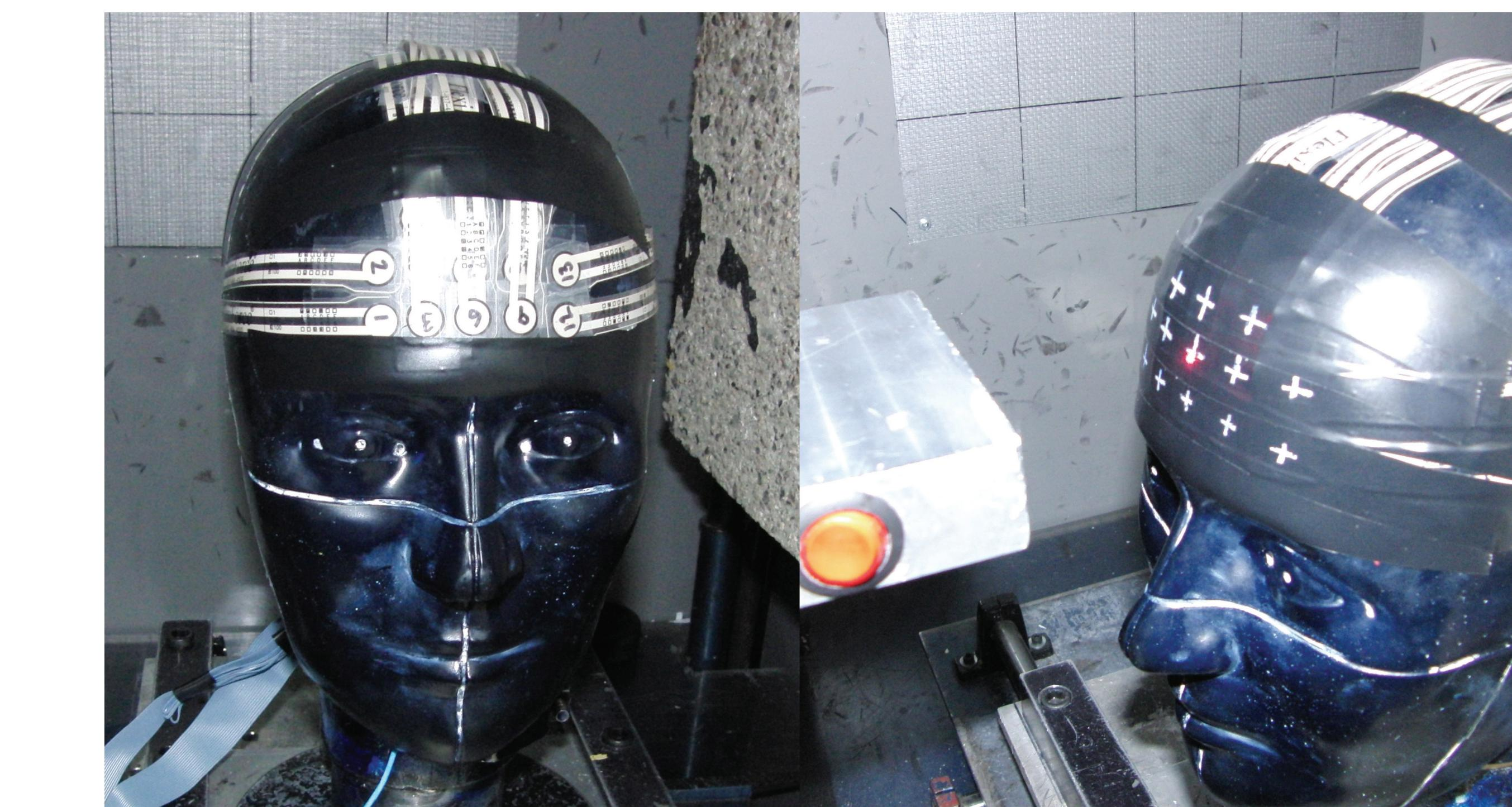
Figure 2: Force sensor array on a NOCSAE full face headform (left) and laser alignment of the puck cannon to the central sensor (right)
