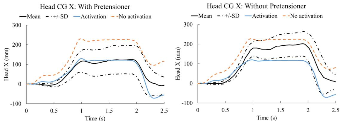
Figure 1: Head CG displacement in the x-direction (forward)
