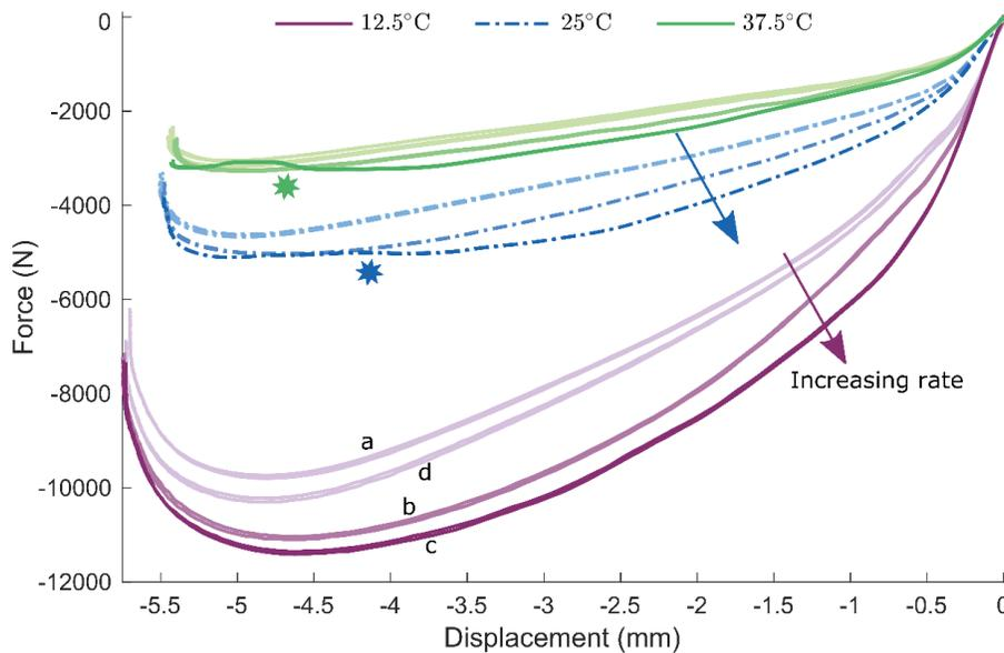
Figure 2. Force-displacement curves for each of the three rates at all three temperatures. Each distinguishable trace includes all repetitions of that test. Colder temperatures and higher rates were associated with increased stiffness. The 12.5°C traces were not repeatable; each letter indicates a pair of tests, applied in the order aa – bb – cc – dd, where a and d represent identical Rate 1 inputs. Star symbols indicate Rate 3 trace regions with marked changes in behavior.
