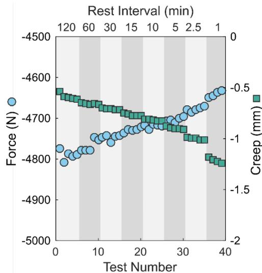
Figure 1. F3mm and creep values from the duration tests. Tests are presented left to right in the order they were run, with bands separating the rest interval levels
