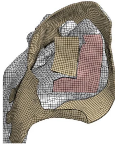
**Figure 2:** Three dimensional finite element representation of the sacroiliac joint (lateral-sacrum view).
