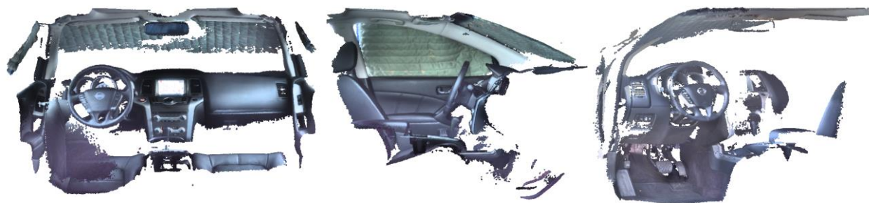
Figure 1. Exemplar vehicle scans from the back-middle seat (left), passenger seat (center), and left door (right) for the Murano reconstruction.
