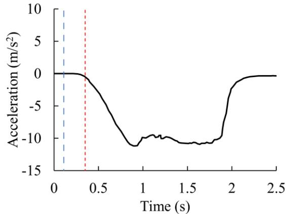
Figure 1: Autonomous braking pulse (Olafsdottir, et al. 2013), the blue line represents activation of pre-tensioner and the red line is for acceleration onset
