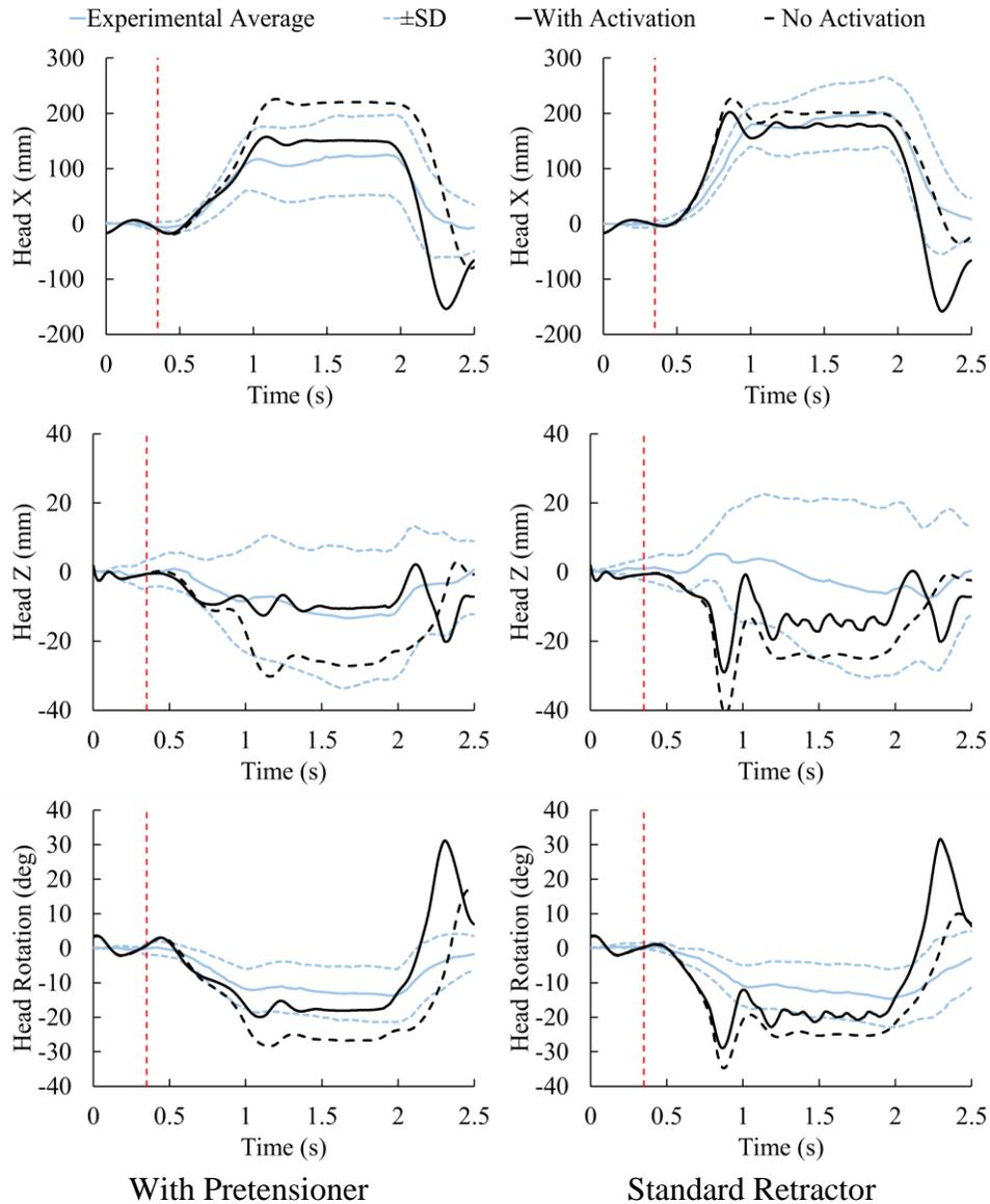
Figure 3: Head CG Kinematics, for simulations with pre-tensioner (left column) and with standard retractor (right column), Vertical dotted red line indicates deceleration onset.
