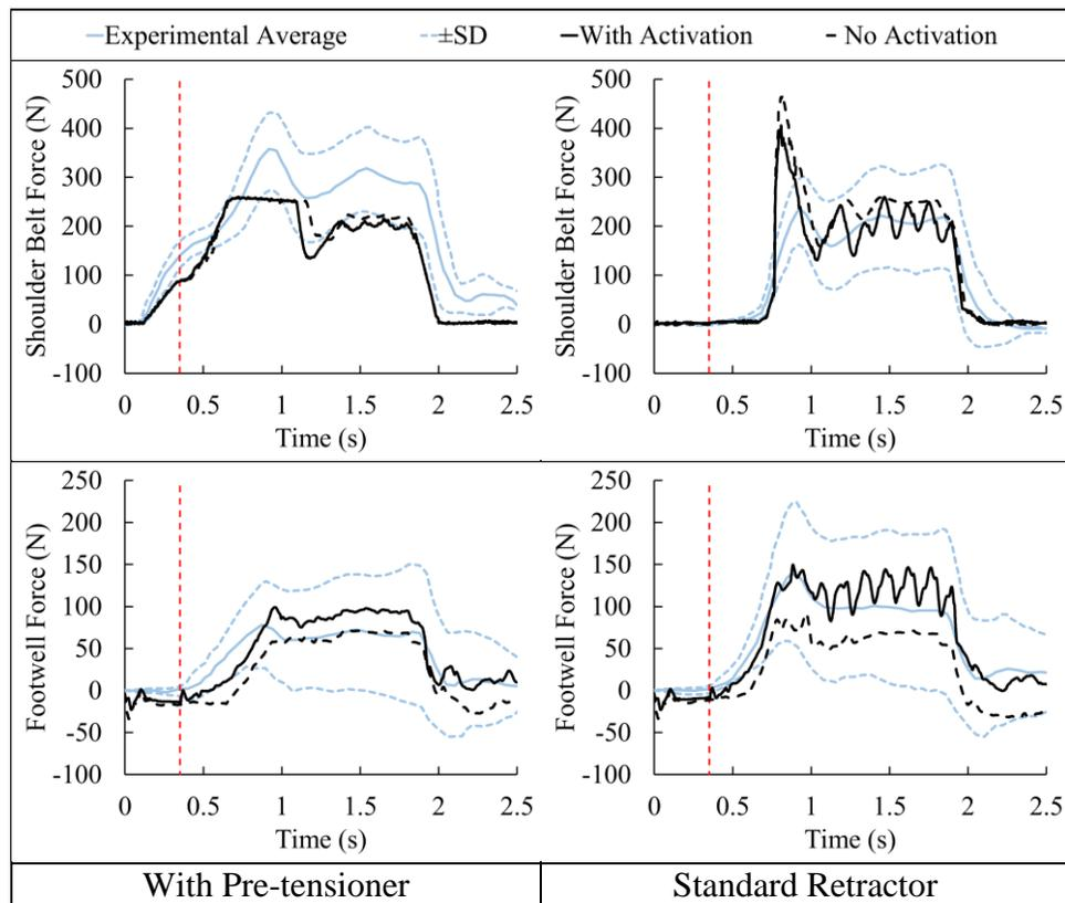
Figure 5: Shoulder belt and footwell forces, for simulations with pre-tensioner (left column) and with standard retractor (right column), Vertical dotted red line indicates deceleration onset.
