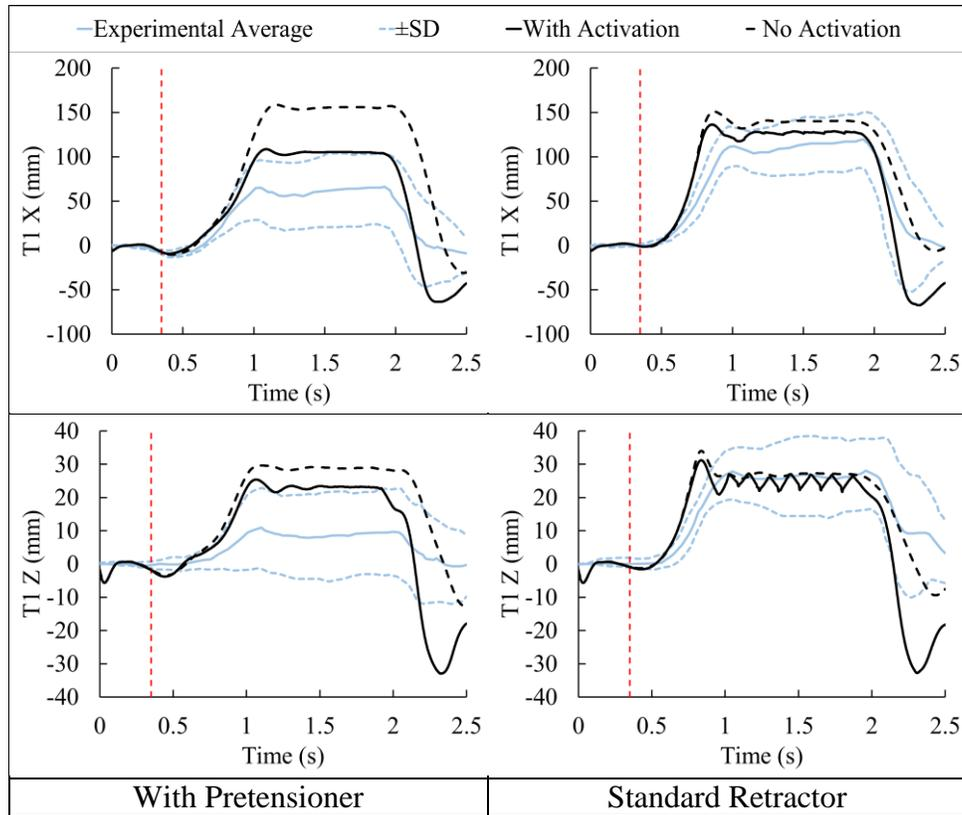
Figure 4: T1 Kinematics, for simulations with pre-tensioner (left column) and with standard retractor (right column), Vertical dotted red line indicates deceleration onset.
