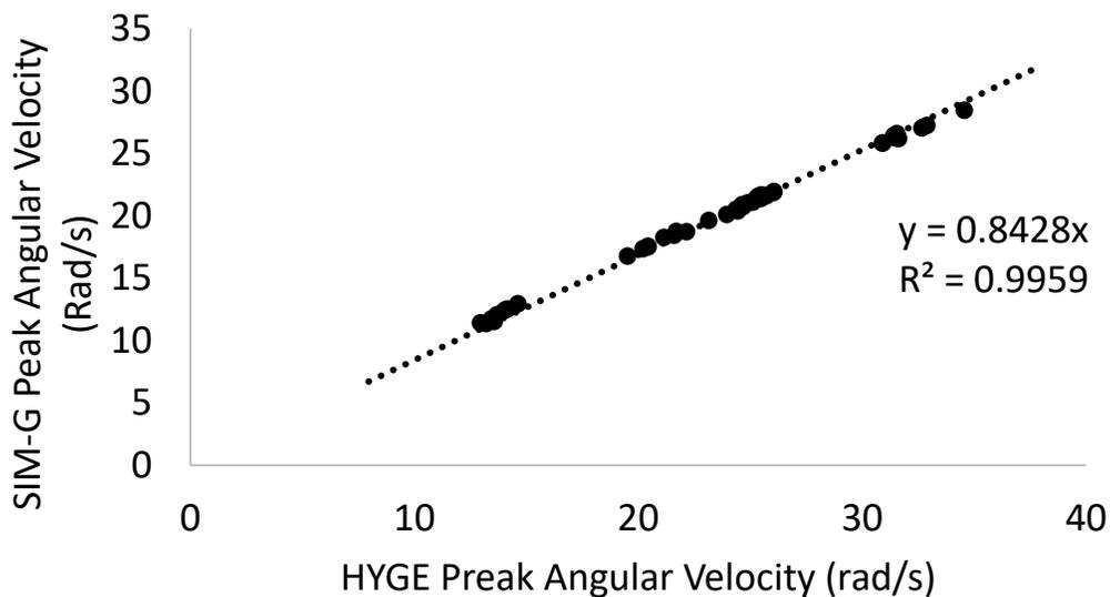
Figure 4. SIM-G peak angular velocity strongly correlates with peak HYPE reference measurements ( $p < 0.001$ ,  $y = 0.8428x$ ,  $R^2 > 0.99$ ).
