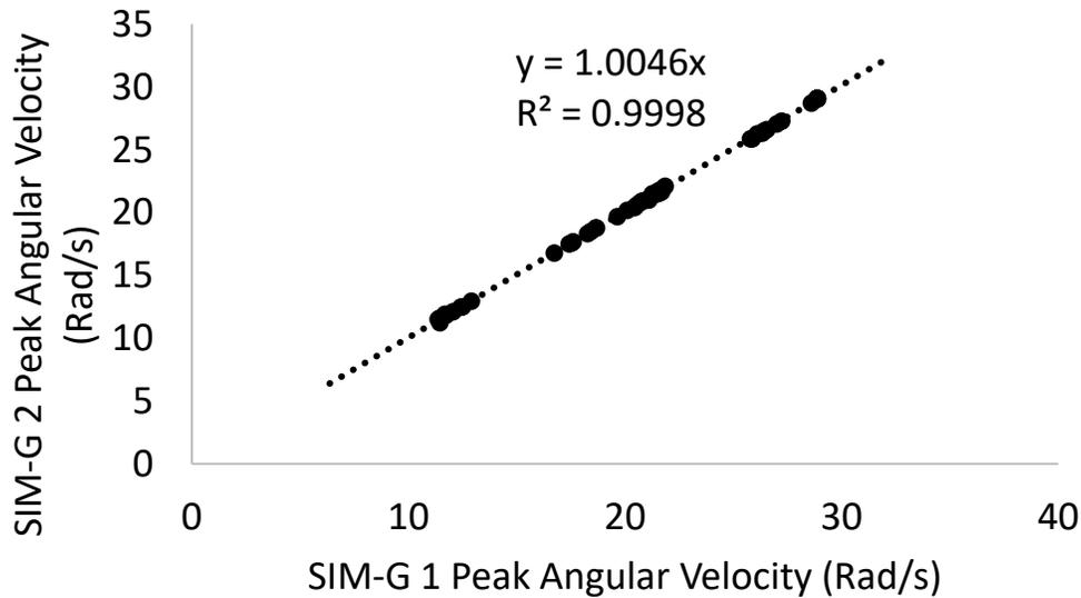
Figure 3: Measurement of peak angular velocity shows strong reproducibility between the pairs of SIM-G sensors subjected to the same angular event ( $n = 2$  pairs of sensors;  $p < 0.001$ ,  $y = 1.0046x$ ,  $R^2 > 0.99$ ). The intercept was set to zero for linear regression.
