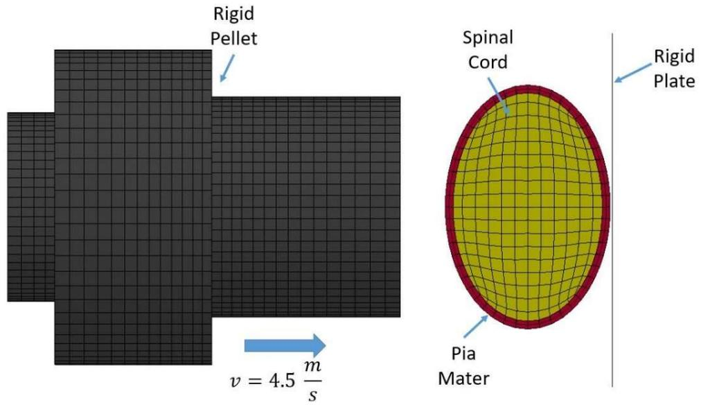
Figure 1. Simulated set up of the dynamic impact on the bovine spinal cord.
