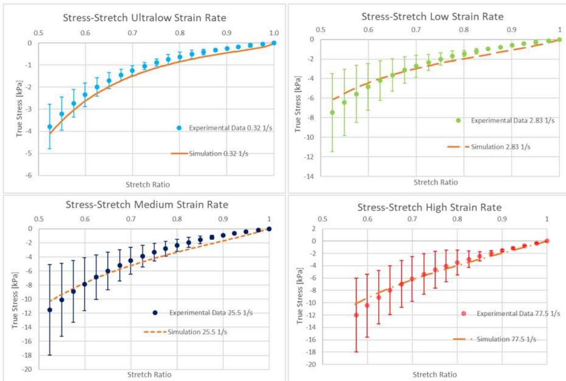
Figure 2. Single element verification of fitted hyper-viscoelastic Ogden model at a given strain rate.
