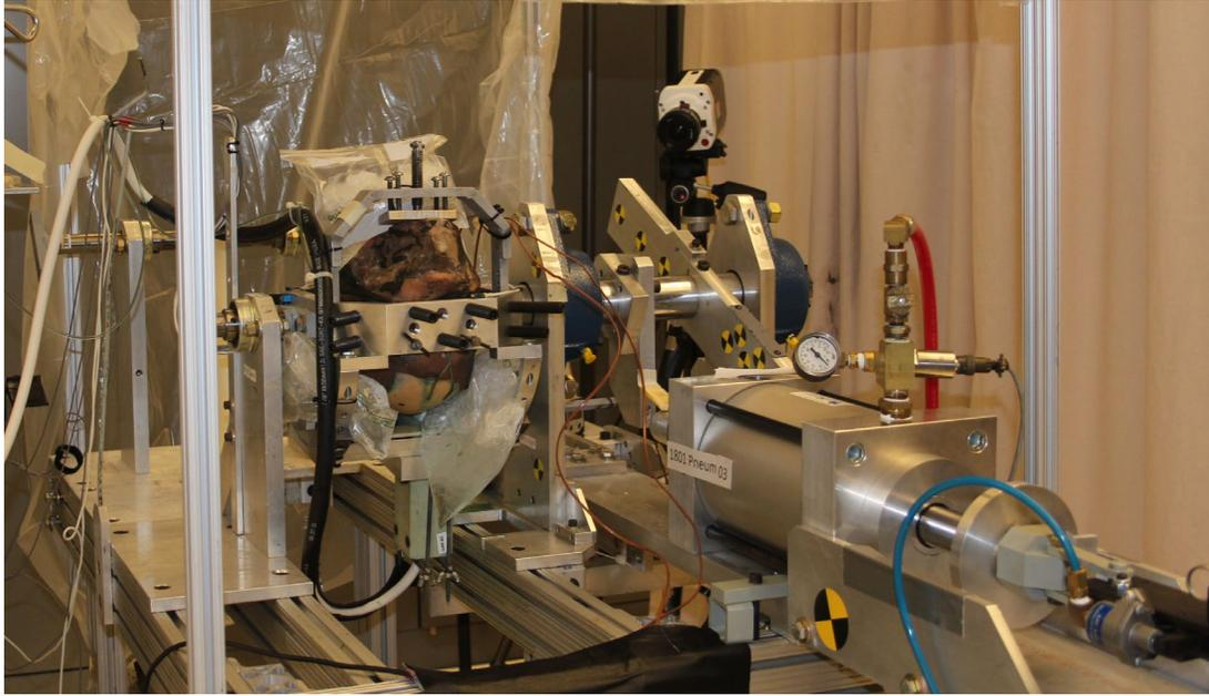
Figure 4: Custom rotation fixture, inverted head in cage (left), pneumatic piston in contact with shaft-mounted loading arm (right)
