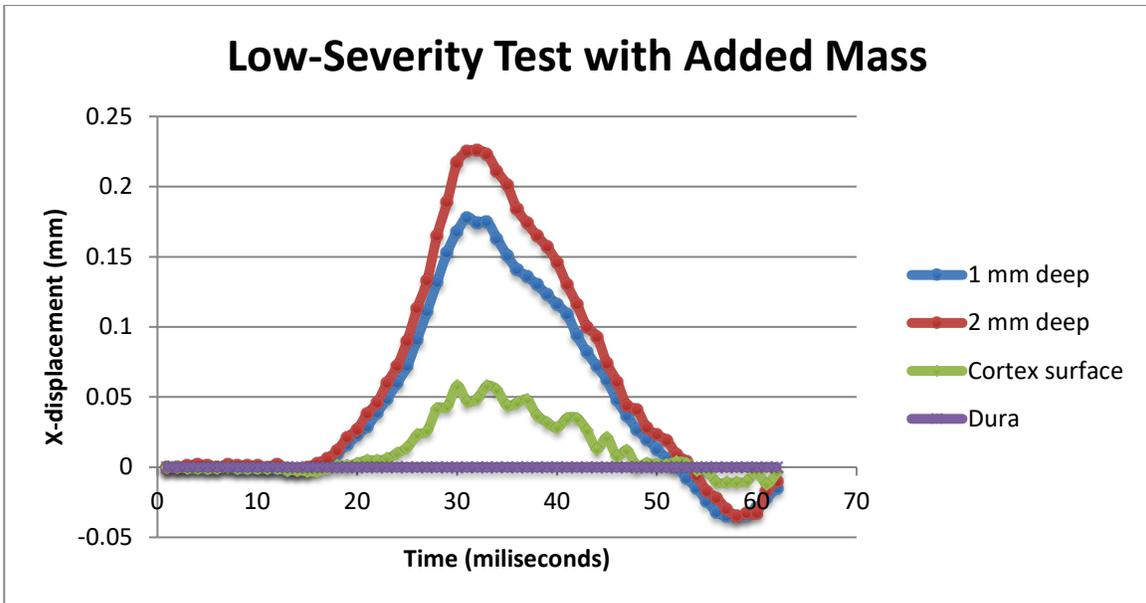
Figure 7: X-displacement relative to skull-mounted ultrasound probe for the low-severity test with added mass
