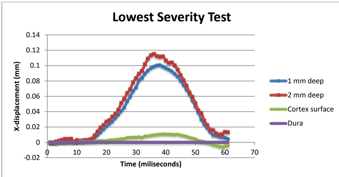
Figure 6: X-displacement relative to skull-mounted ultrasound probe for the lowest severity test analyzed
