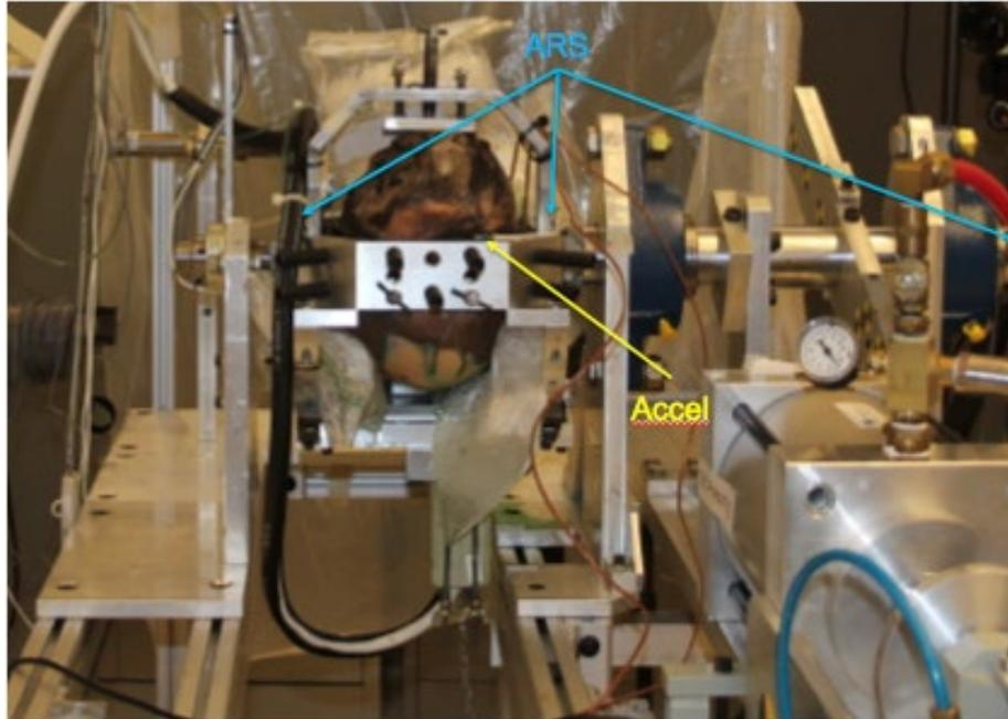
Figure 5: Fixture-mounted instrumentation locations
