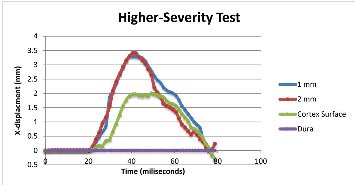
Figure 8: X-displacement relative to skull-mounted ultrasound probe for the 50 PSI pneumatic test
