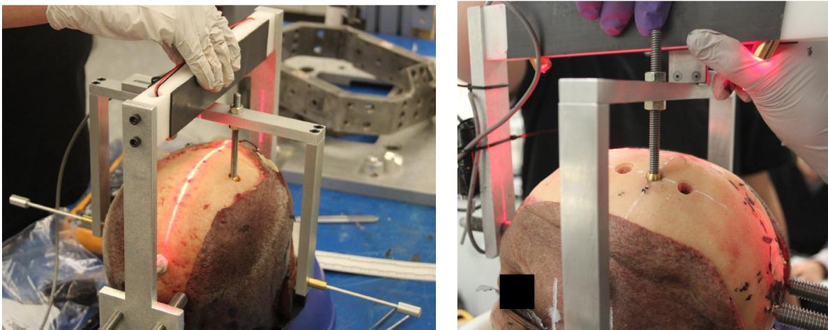
Figure 2: Head Alignment Tool (HAT)
