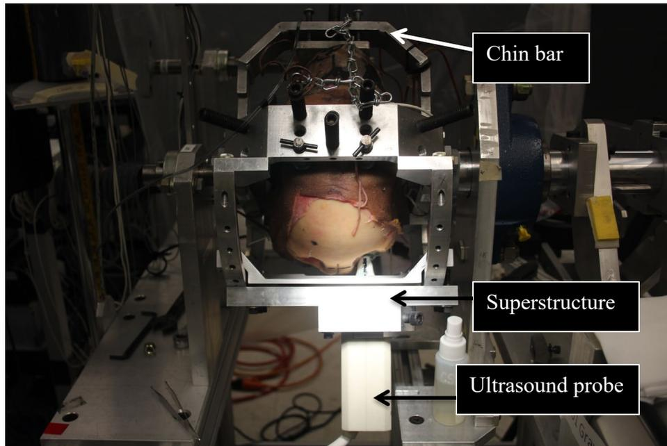
Figure 3: Head in cage installed in rotation fixture with chin bar at top, ultrasound probe mounted in superstructure at bottom
