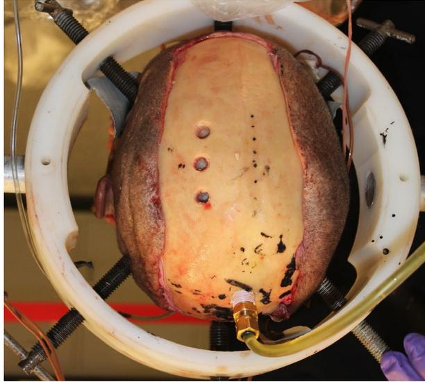
Figure 1: SSS (bottom, with plumbing inserted) and transducer holes before grinding (left of centerline)
