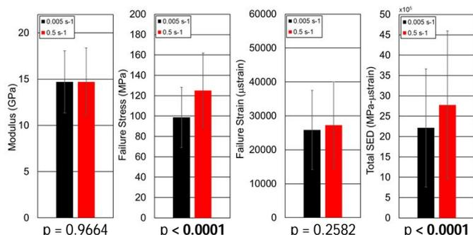
Figure 2. Comparison of modulus (left), failure stress (left-center), failure strain (right-center) and total SED (right) between 0.005 strain/s and 0.5 strain/s.
