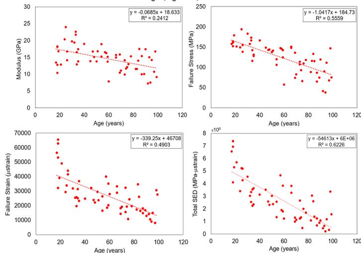
Figure 3. Modulus versus age (top left), failure stress versus age (top right), failure strain versus age (bottom left), and total SED versus age (bottom right) at 0.5 s<sup>-1</sup>.
