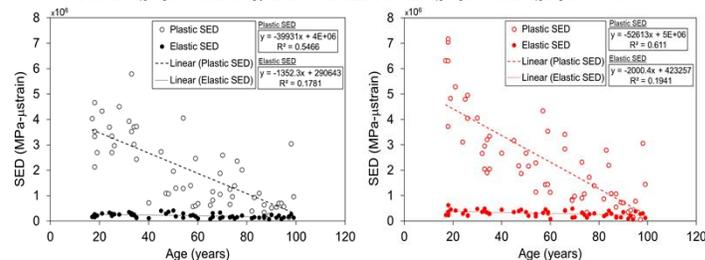
Figure 4. Plastic and elastic strain energy density versus age at 0.005 s<sup>-1</sup> (left) and 0.5 s<sup>-1</sup> (right).
