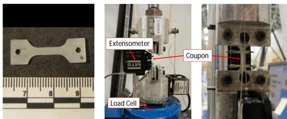
Figure 1. Final dog-bone coupon (left), frontal view of experimental set-up with clamped coupon (center), and side view of experimental set-up (right).
