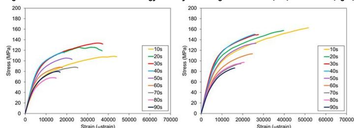
Figure 5. Characteristic average curves for 0.005 s<sup>-1</sup> tests (left), and 0.5 s<sup>-1</sup> tests (right) for each decade.
