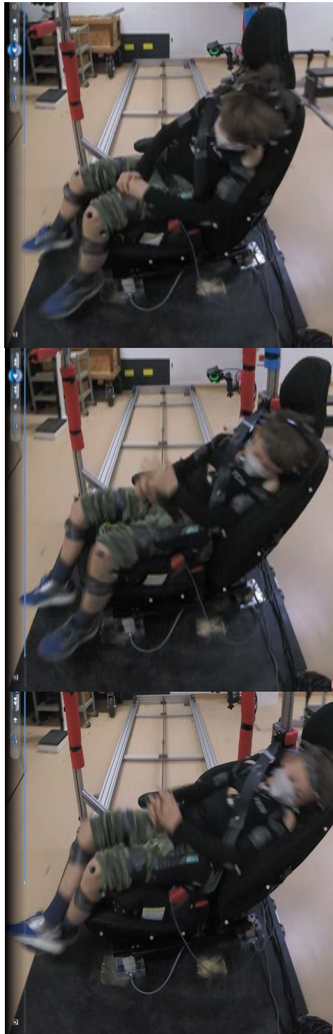
Figure 6: Side view of head and trunk displacement at seatback recline angles of 25°, 45°, 60° (top to bottom)
