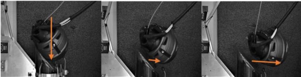
Figure 3: Representative impact sequence for the high COF surface (80-grit sandpaper), where the helmet bounces off the anvil spinning clockwise, and the low-COF surface (steel), where the helmet rolls off the anvil spinning counter-clockwise.
