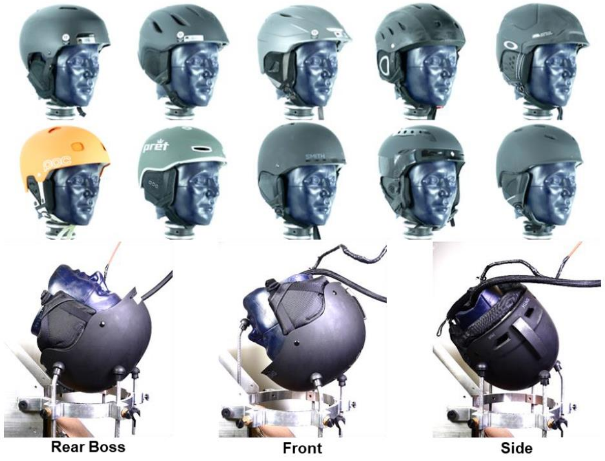
Figure 1: Ten helmet models tested and the three impact locations.
